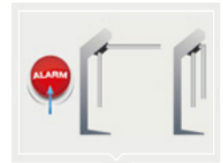
Turnstiles folding arms can be released by alarm button
